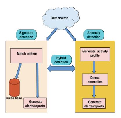
**Figure 5.** Detection methods utilized by intrusion detection system (Madhavi, 2015)
