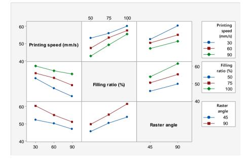
Figure 3. Bending strength changes according to production parameters.
