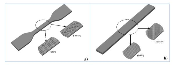
Figure 1. Sample 3D models; a) Tensile, b) Bending
