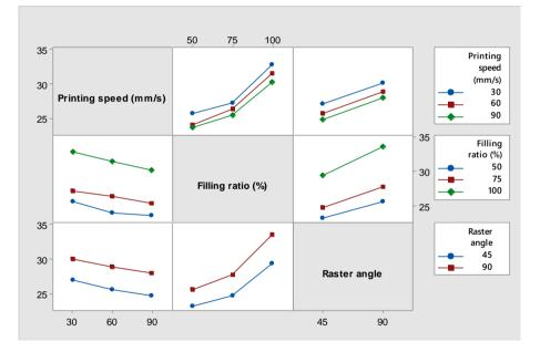
Figure 2. Tensile strength changes according to production parameters
