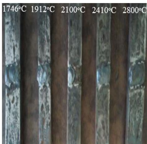
**Fig. 2.** Welded Samples showing Welding Temperatures
