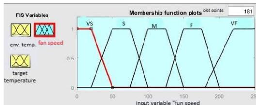
**Figure 2.** Fan speed membership functions valuation. VS= [-25 0 25 50], S= [25 50 75 100], M= [75 150 125 150], F= [125 150 175 200], VF= [175 200 225 260]
