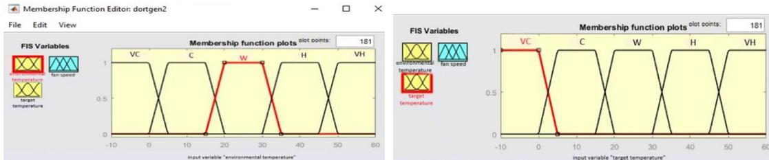
**Figure 1.** Environmental temperature and Target temperature membership functions valuation. VC= [-20 -10 0 5], C= [0 5 15 20], W= [15 20 30 35], H= [30 35 45 50], VH= [45 50 60 70]
