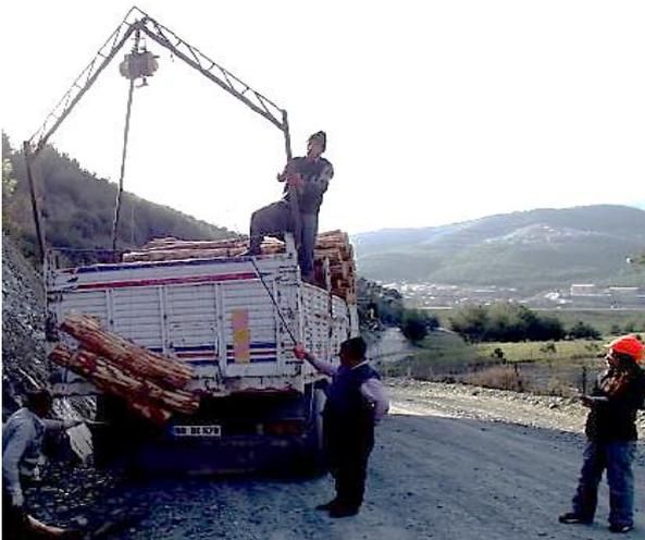
Figure 3. Electric powered winch loading
