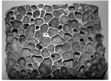
Figure 3. Aluminium based foam material
