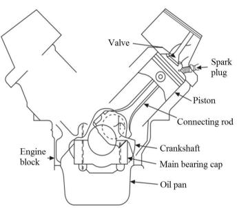
Figure 8. Schematic representation of the piston motor
