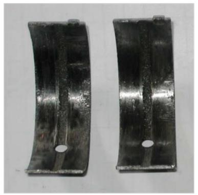
Figure 22. Crankshaft master bearings coated by FSM using a new alloy of Pb, Sn, Cu and ZrO<sub>2</sub> powders
