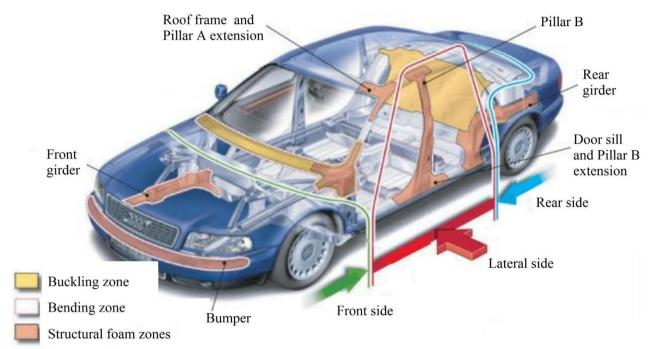
Figure 18. Structural foam materials used on Audi A8
