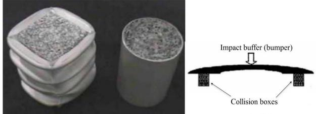
Figure 20. Collision boxes used in automobiles
