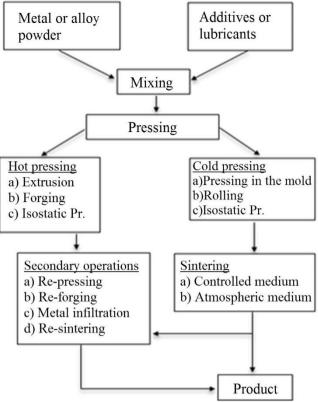
Figure 1. Flow diagram for parts production with PSM
