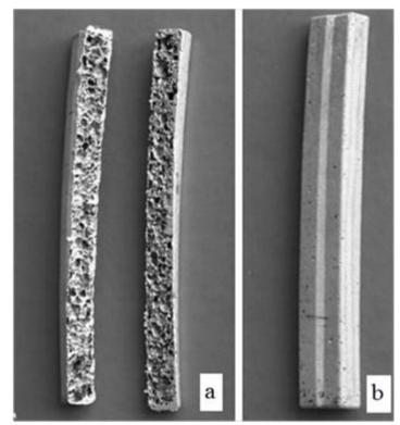
Figure 19. A-column in automobiles: a) made from Al foam, b) made from steel sheet
