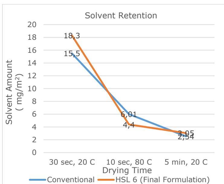
**Figure 12:** Residual solvent amounts [mg/m<sup>2</sup>].
