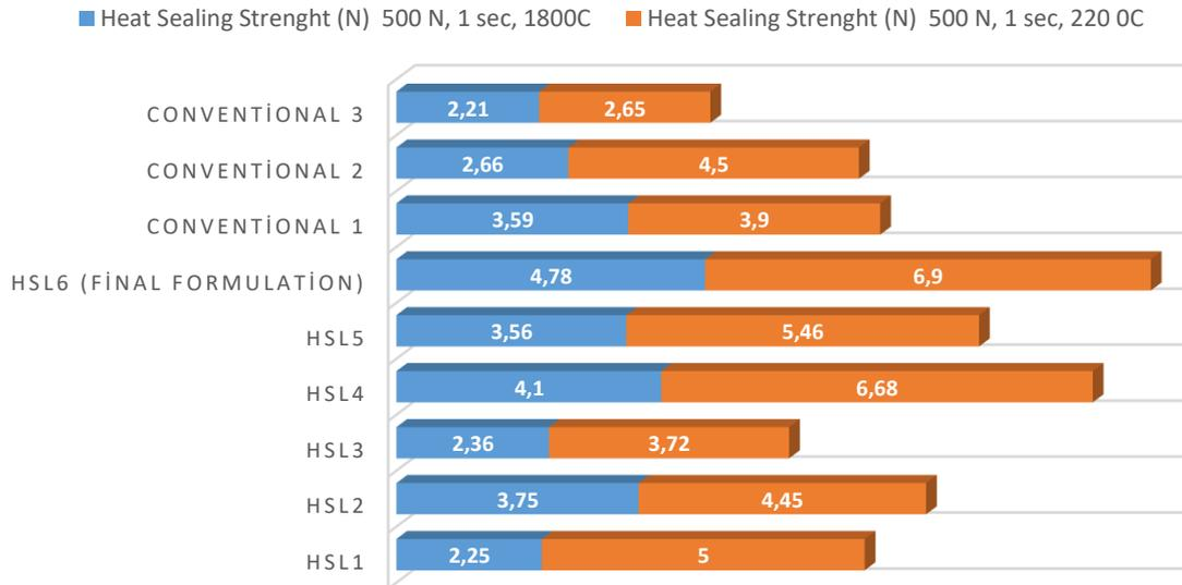
Figure 6: HS Strengths in Newton at sealing condition 1 and 2.
