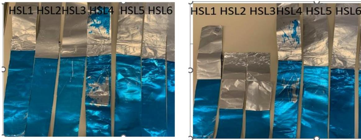
**Figure 11:** Block Test Result of Drawdowns at conditions 45 °C, 3 days, 45 kg & 20-25 °C, 1 week, 10 tons.
