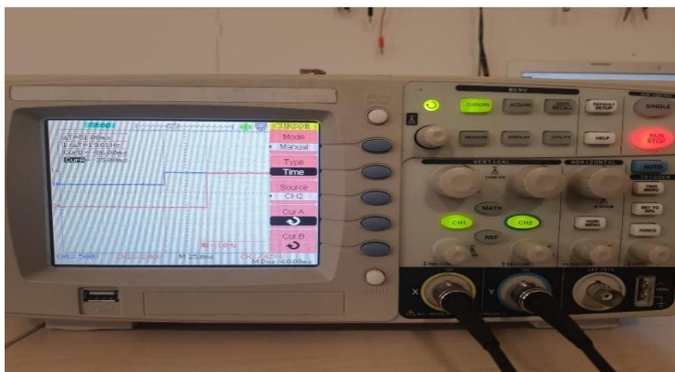
**Figure 10.** Experimental time delay result for Arduino circuit
