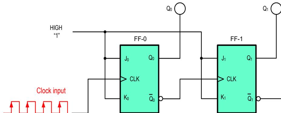
**Figure 2.** Two-bit asynchronous binary up counter
