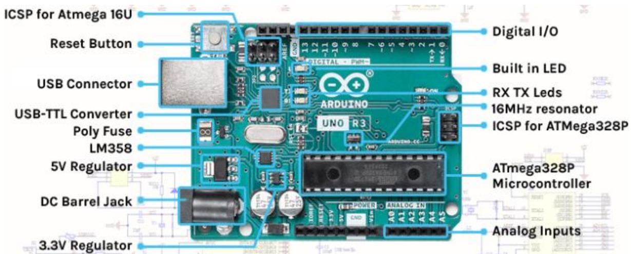
Figure 4. Labeled diagram of an Arduino Board
