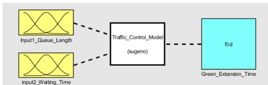
Figure 8. Fuzzy logic control for intelligent traffic
