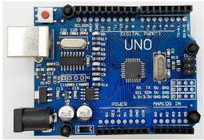
Figure 4. Arduino Uno microcontroller board
