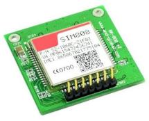
Figure 9. SIM808 GSM modem
