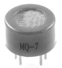
Figure 6. MQ7 air quality sensor
