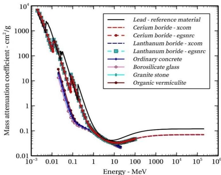
**Figure 7.** Comparison of the mass attenuation coefficients of lanthanumhexaboride and ceriumhexaboride with some other standard shielding materials (lead, granite, vermiculite, borosilicate and concrete) [36,39,40].
