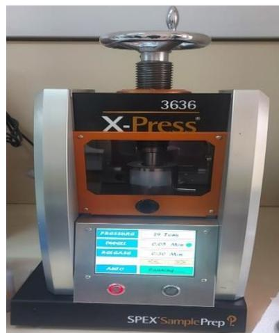
**Figure 2.** Press machine with 30 tons capacity.
