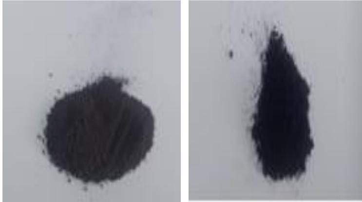
**Figure 1.** Appearance of LaB<sub>6</sub> and CeB<sub>6</sub> powder samples.
