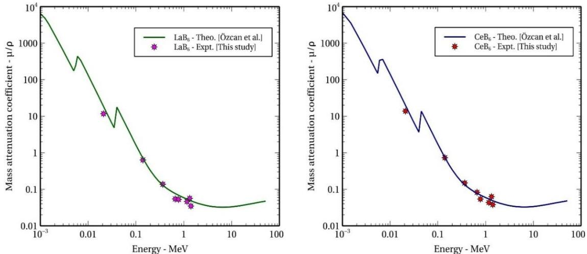
**Figure 6.** Comparison of the experimental data with the previous theoretical simulation results [37] for lanthanumhexaborides and ceriumhexaboride.
