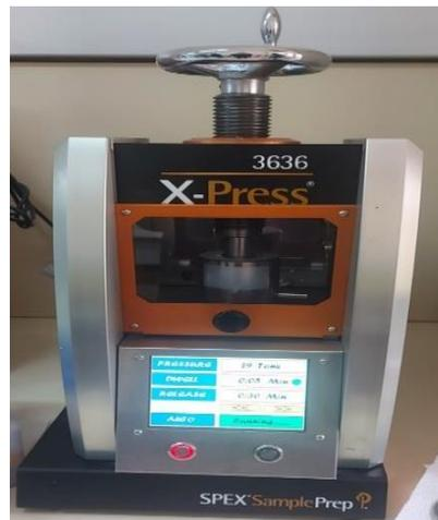
**Figure 2.** Press machine with 30 tons capacity.
