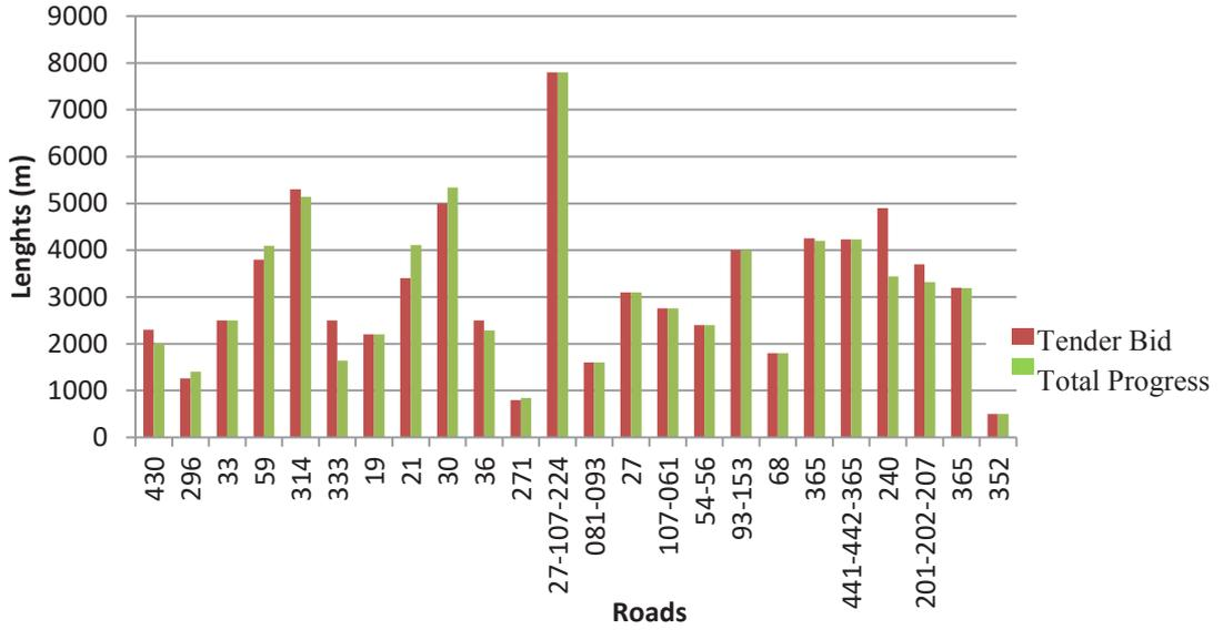
Figure 4. Differences chart between tender bid and total progress road lengths
