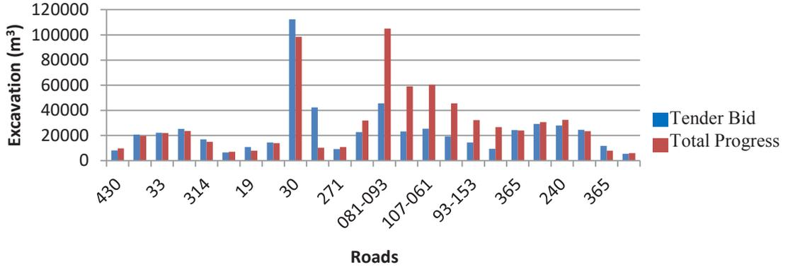
Figure 3. Differences chart between tender bid and total progress excavation among
