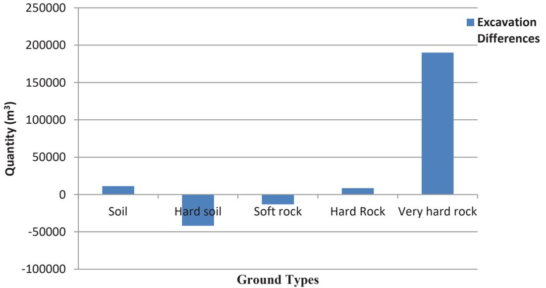
Figure 5. According to excavation classes, differences chart between tender bid and the total progress excavation among
