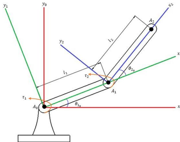
**Figure 1:** Two degrees of freedom robot arm.
