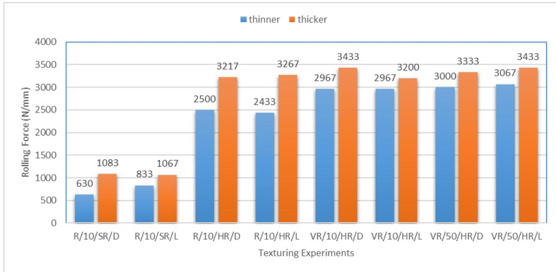
**Figure 6.** The material thickness effect on rolling force
