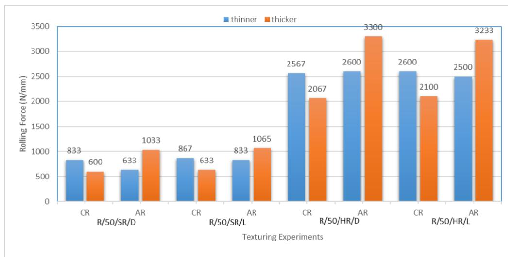
**Figure 7.** Comparison of rolling force in CR and AR based on material thickness reduction (CR data is taken from the other article (Çolak & Kurgan, 2018))
