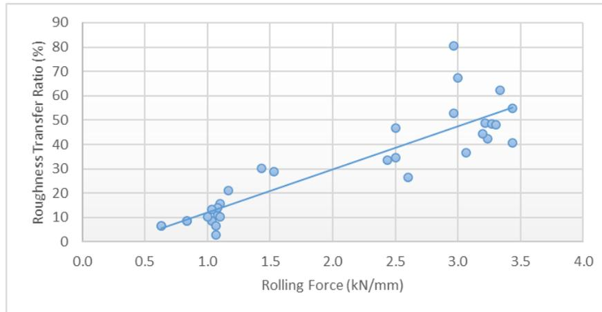
**Figure 5.** The rolling force effect on RTR
