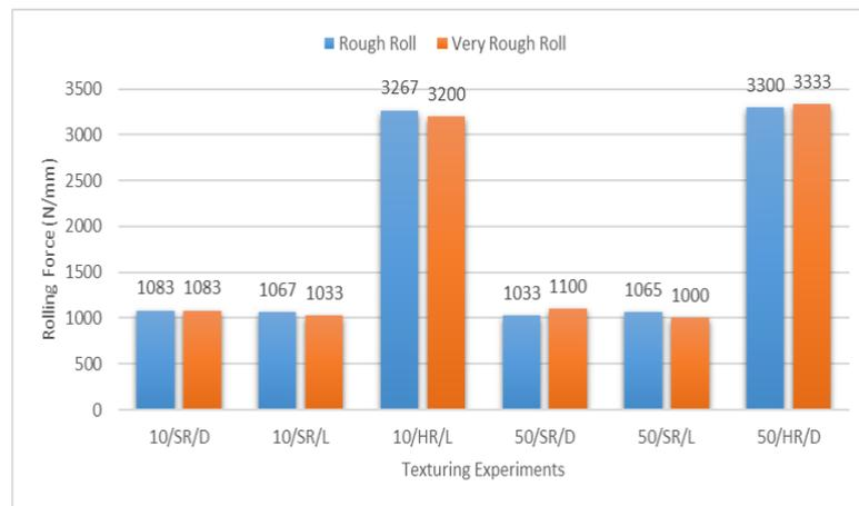
**Figure 10.** The roll roughness effect on the rolling force (for thicker material)
