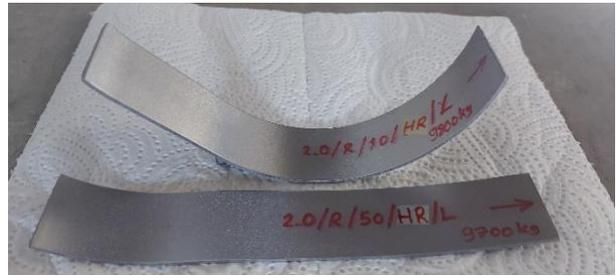
b) The speed effect on material curvature.
