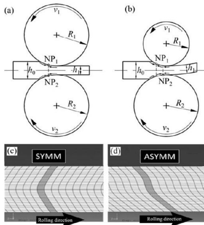
**Figure 1.** Schematic illustrations **a)** Symmetric rolling ( $R_1=R_2$ ,  $V_1=V_2$ ) **b)** Asymmetric rolling ( $R_1<R_2$ ,  $V_1<V_2$ ) **c)** Shear deformation texture through the thickness in CR **d)** Heterogeneous shear deformation texture through the thickness in AR (Liu & Kawalla, 2012).
