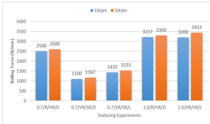
**Figure 8.** The speed effect on rolling force
