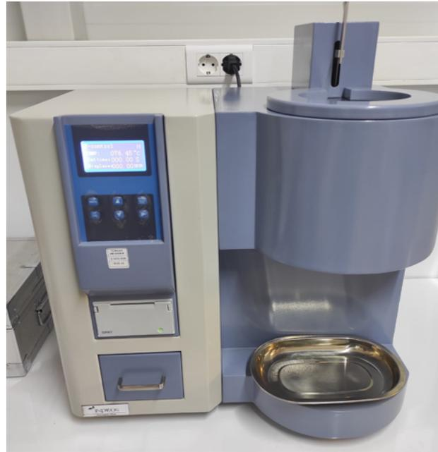
Figure 7. Melt flow index test of polymers
