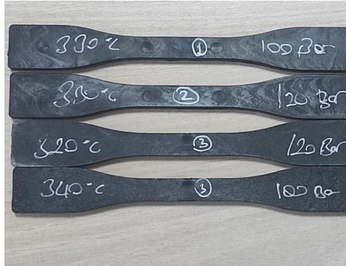
Figure 2. Tensile test specimens for PPS
