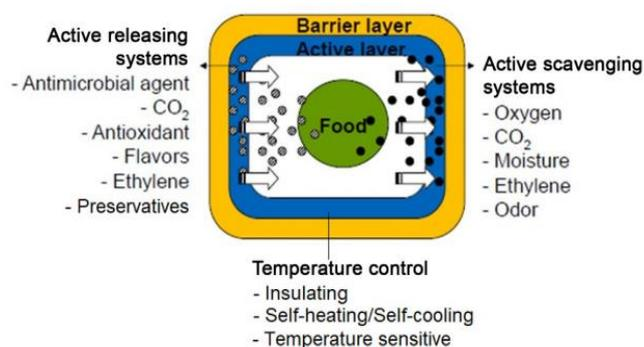
**Figure 2.** The active packaging system (Kuswandi and Jumina, 2020)
