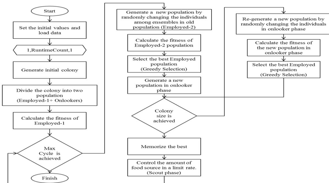
Figure 5. Flow chart of the proposed algorithm
