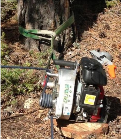
Figure 3. Installation of portable winch on a standing tree
