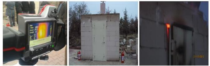
Figure 2. The experiment images of the fire door
