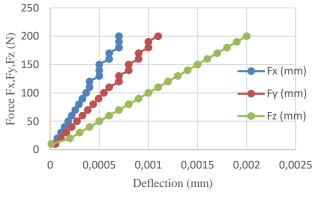
**Figure 3.** Force-deflection curve for  $F_x$ ,  $F_y$ ,  $F_z$
