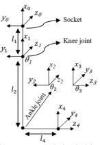
Figure 2. The coordinate systems attached to the joint
