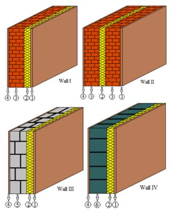
①External plaster ②Insulation ③Brick ④Internal plaster ⑤Concreta ⑥CSEB
