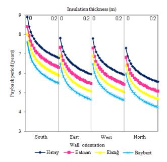
Figure 9. Effect on payback period of insulation thickness and different orientations for sandwich wall insulated with extruded polystyrene and selected cities.
