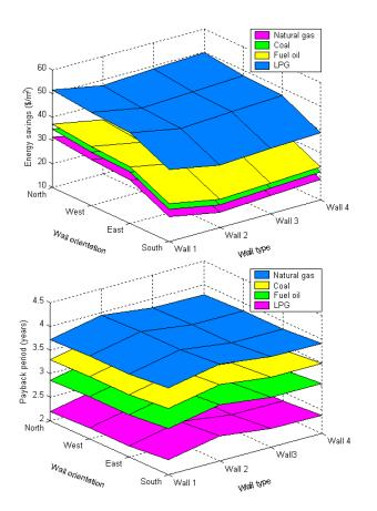
Figure 7. Variation of energy savings and payback period with different wall structures and orientations for different fuel types and extruded polystyrene insulation material in Elazığ
