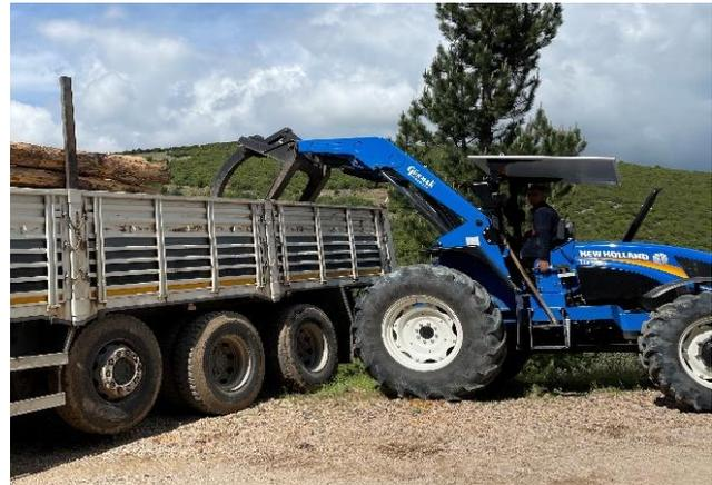
Figure 3. Loading operation with tracked loader (Sumitomo SH135) (left) and rubber-tired loader (New Holland TD 90D) (right)
