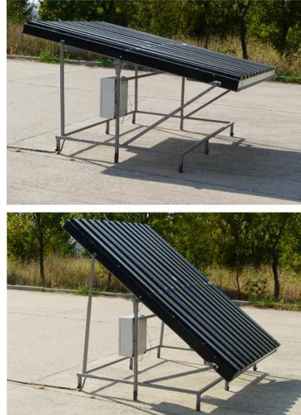
**Figure 4.** The 5 m<sup>2</sup> experimental setup used for roof ventilation measurements
