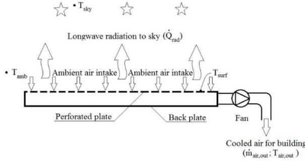
**Figure 5.** Physical model of nocturnal radiative air cooling with a transpired solar collector
