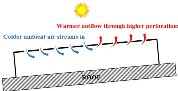
**Figure 3.** Natural ventilation in a roof mounted TSC
