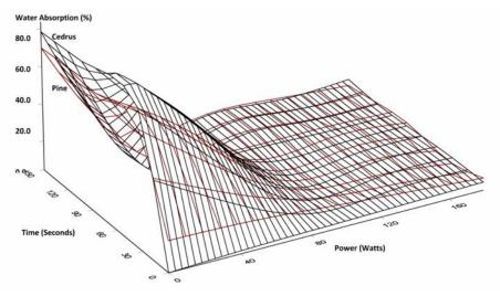
Figure 4. The water absorption (%) properties of MW treated softwoods.
