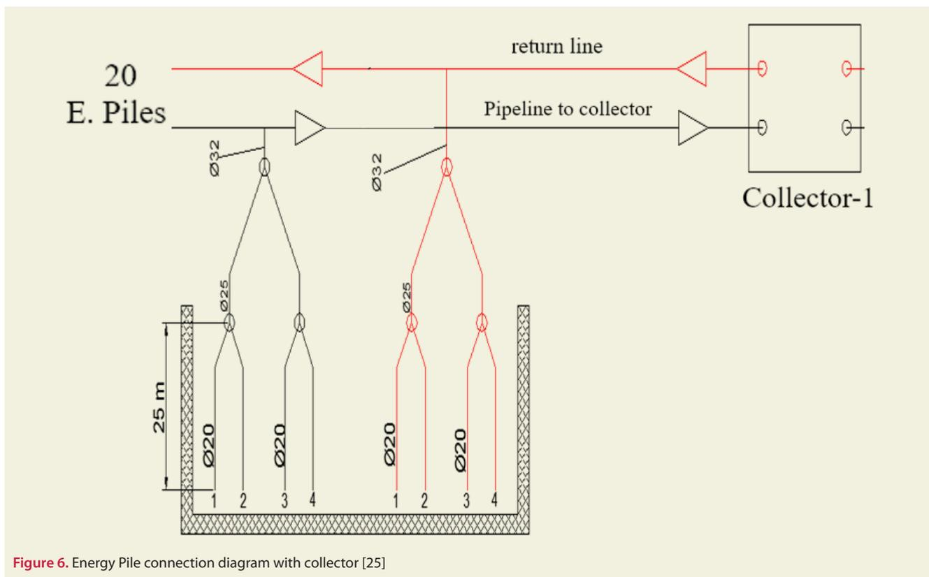
Figure 6. Energy Pile connection diagram with collector [25]
