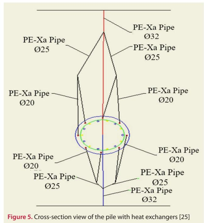
Figure 5. Cross-section view of the pile with heat exchangers [25]
