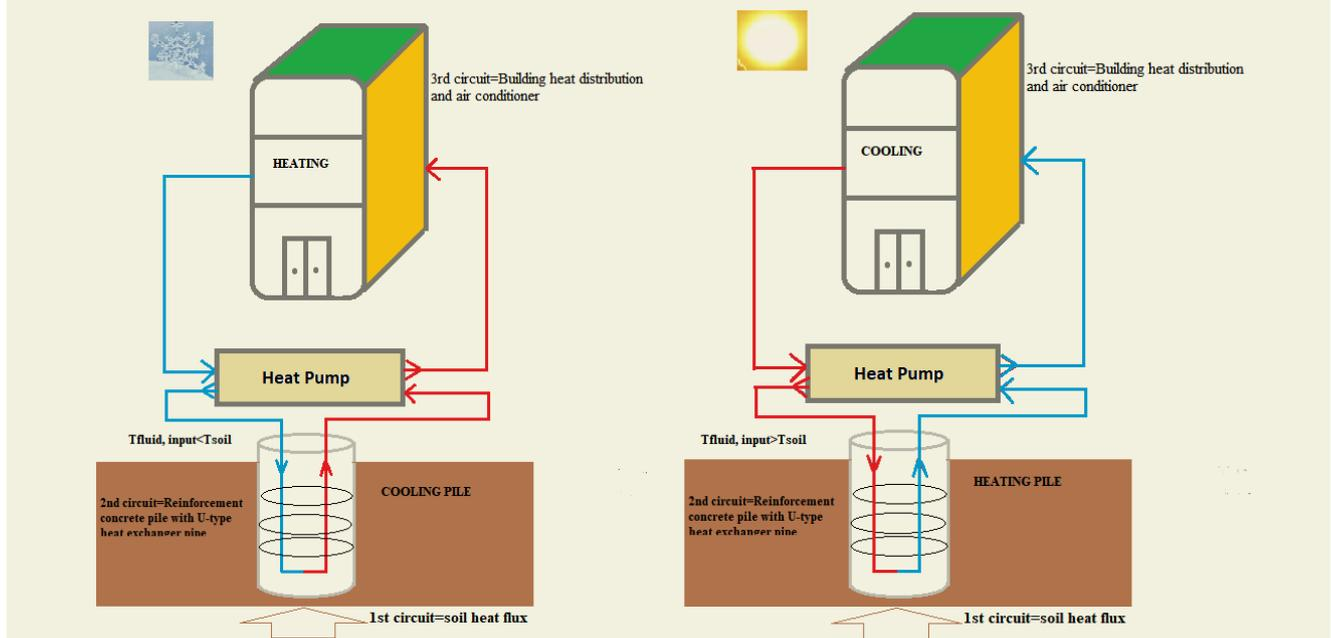
Figure 2. a) Energy extraction b) Energy storage
