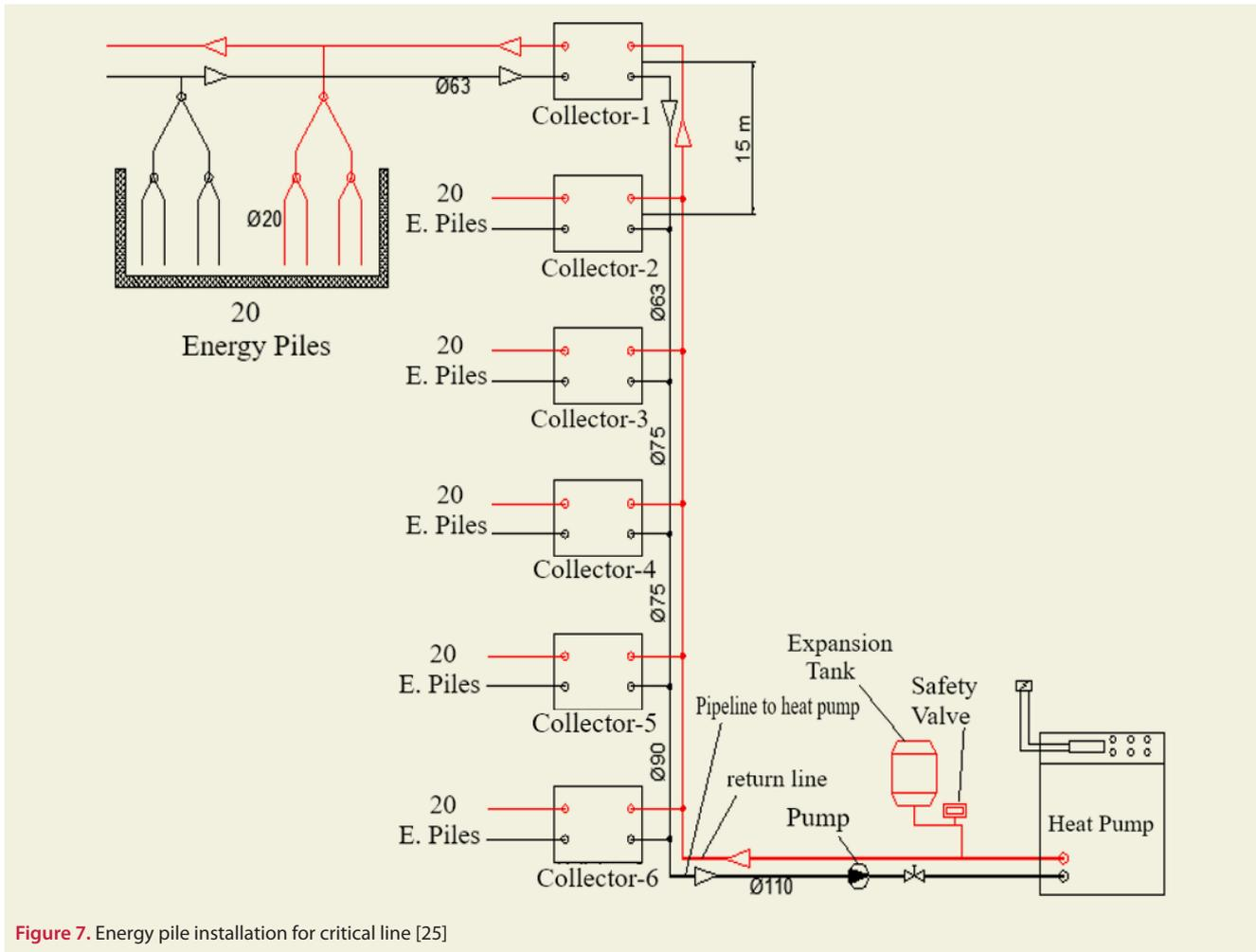
**Figure 7.** Energy pile installation for critical line [25]
