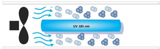
Figure 3. Ozone formation by Ultraviolet method [29]
