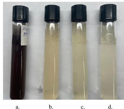
**Figure 7.** Ozonated samples: a. initial wastewater b. 10 min ozonated wastewater c. 20 min ozonated wastewater d. 30 min ozonated wastewater
