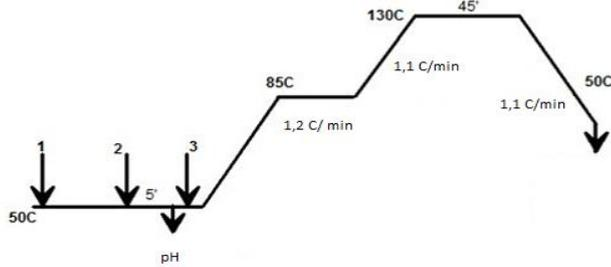
**Figure 4.** Dyeing diagram
