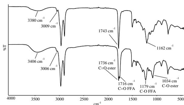
**Figure 4.** FTIR spectra of castor oil and product
