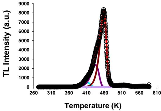
Fig.2 CGCD of the TL glow curves for LiF (at 5%) at pre-heat temperature of 140°C.
