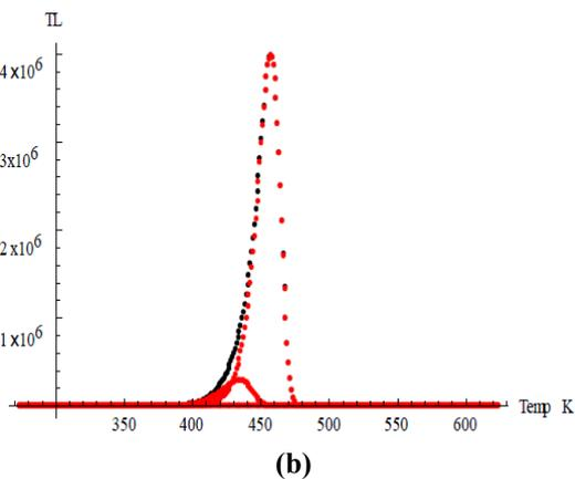
**Fig. 5** Simulation results of the thermal fading at 140°C with:  $E_3=1.4$  eV;  $T_{m3}=409$ K;  $E_4=1.5$ eV;  $T_{m4}=434$ K;  $E_5=2.15$ eV;  $T_{m5}=457$ K respectively.
