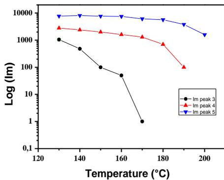
Fig.4 Maximum TL intensity dependence on pre-heat temperature.
