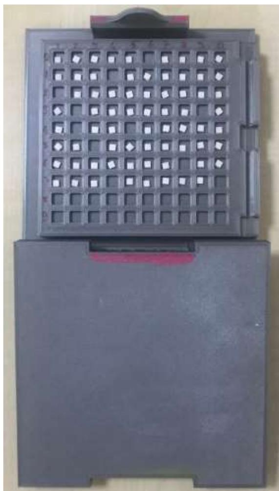
**Figure 6.** A printed version of the TLD holder cassette
