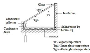
Figure 4. Solar still with internal heat exchanger [18].
