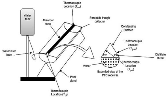
Figure 12. Schematic of the test setup.
