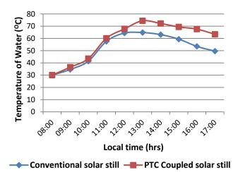
Figure 14. Comparative analysis of Conventional and PTC Coupled Solar Still.
