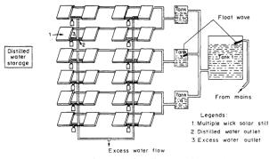
Figure 1. Multi wick distillation plant [10].
