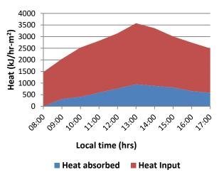
Figure 16. Heat input and absorbed for conventional solar still.
