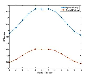
Figure 9. Optical and Thermal efficiency of the PTC System (Theoretical Modeling).
