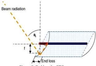
Figure 8. End loss for PTC system.
