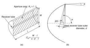
Figure 7. Geometry of the Parabola [45].
