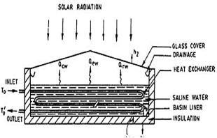
Figure 3. Solar still with internal heat exchanger [16].
