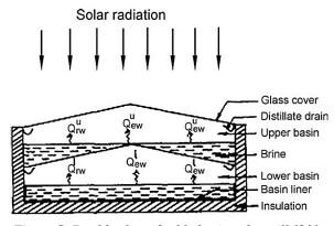
Figure 5. Double slope double basin solar still [23].
