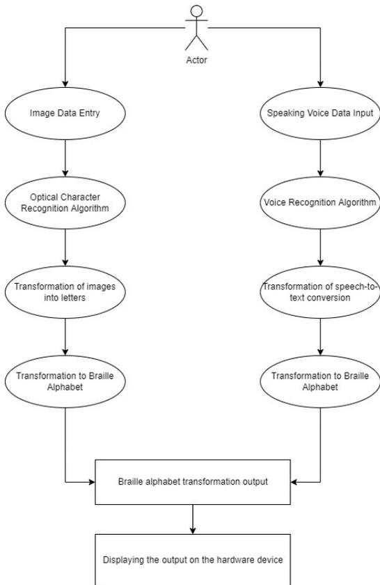
**Figure 1.** Unified Modelling Language(UML) Diagram of Conversion Project to Braille Alphabet with Optical Character Recognition (Algorithm 1) and Voice Recognition Algorithm (Algorithm 2).
