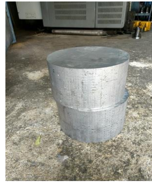
Fig.7 Aluminum blocks before being processed into two hemispheres of the chamber system
