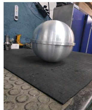
Fig.9 Post-CNC manufacturing, basic spherical geometry reached
