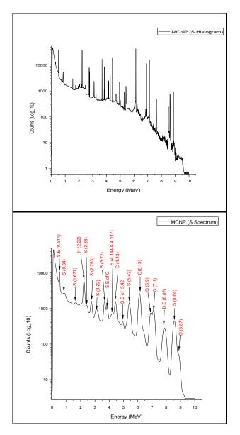
Fig.11 MCNP5 Histogram and spectrum of S element.
