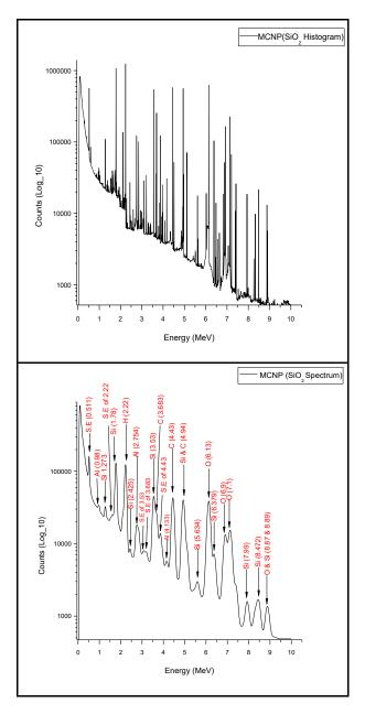
*Fig.8 MCNP5 Histogram and spectrum of* SiO<sub>2</sub> *compound.*
