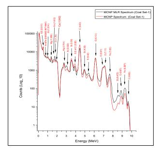
*Fig.12* Comparison the MCNP5 Spectrum of Coal Set-1 with Coal Set-1 spectrum obtained from MLR method.
