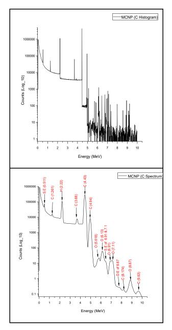
Fig.9 MCNP5 Histogram and spectrum of the Carbon element.
