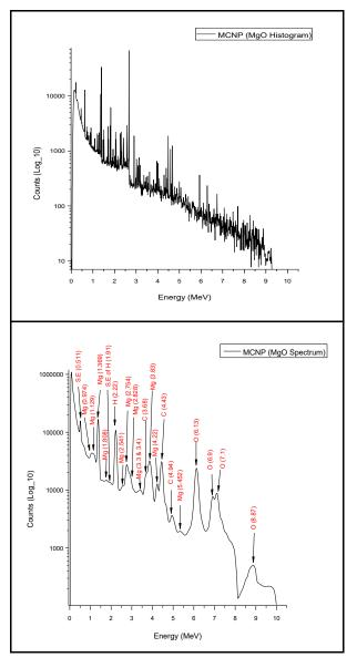
*Fig.10 MCNP5 Histogram and spectrum of MgO compound.*
