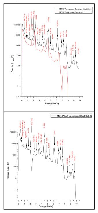
Fig.2 MCNP5 gamma rays spectrum of Coal Set-1.
