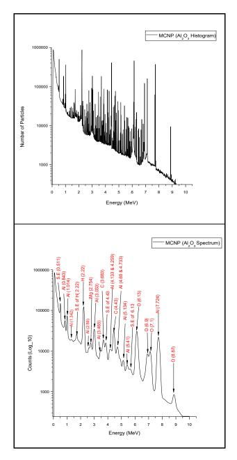
*Fig.5 MCNP5 Histogram and spectrum of Al*<sub>2</sub>*O*<sub>3</sub> *compound.*
