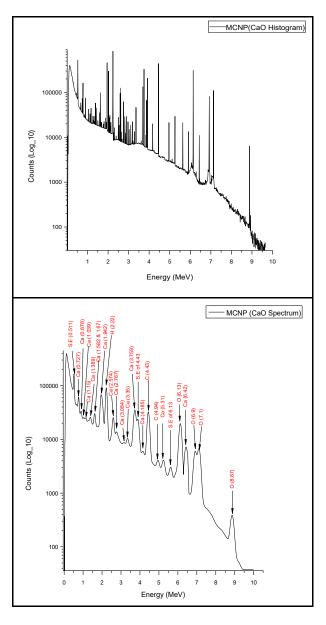
Fig.6 MCNP5 Histogram and spectrum of CaO compound.
