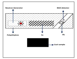
Fig.1 The schematic view of the MCNP5 simulation geometry.
