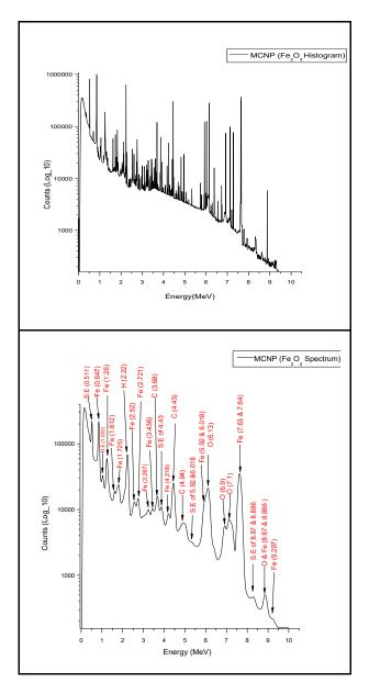
Fig.7 MCNP5 Histogram and spectrum of Fe<sub>2</sub>O<sub>3.</sub>
