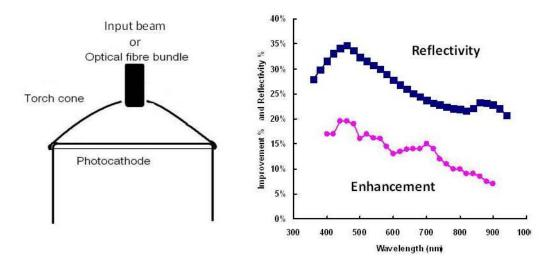
*Fig.1* Addition of a torchlight reflector reduces losses from the reflections of the high refractive index photocathode. In an initial test the gains were up towards 20%.
