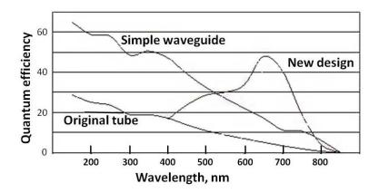
Fig.3(b) Examples of sensitivity enhancements produced by using waveguiding techniques, data are compared with normal head on illumination of the same S20 PM tube
