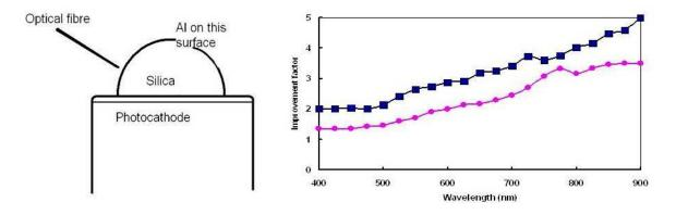
*Fig.2* By using high angles of incident light there is enhanced absorption in the photocathode. In these trials, with different S20 tubes, improvements of up to 5 times appeared at long wavelengths.
