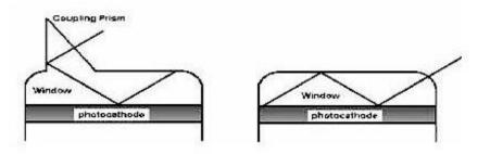
Fig.3(a) Two routes for using the benefits of waveguiding in the window of the PM tube.
